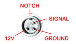
The best way to alter the chiller for use with 3rd party temperature controllers is to create a wiring adapter that will be compatible with the chiller's M12 connections. This can be done by using a relay to form a connection between the M12, 12V and ground pins. The relay can be controlled by the temperature controller cooling output signal. The specific requirements depend on the temperature controller in question.
